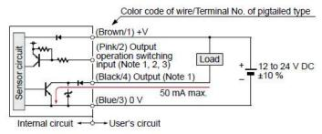
Notes: 1) The emitter of a thru-beam type does not incorporate output (black/4) and output operation switching input (pink/2).
