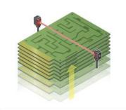
Determining cutting position of sheet
